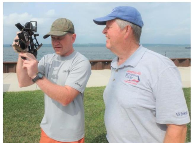
Figure 33: Bring the sun's lower edge down to the horizon and read the angle. Bill Trondsen and Jim McGinnis.
